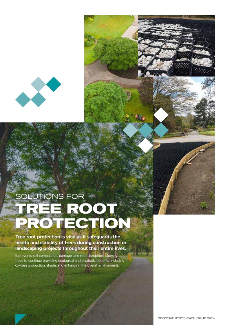
Geocells and geotextiles offer a holistic solution that not only ensures the durability and stability of the path, road or car park, but also safeguards the health and vitality of nearby trees, particularly their intricate root systems.
